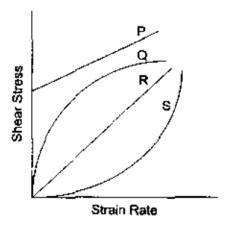
The most suitable relation for flow of tooth paste being squeezed out of the tube is given by the curve
